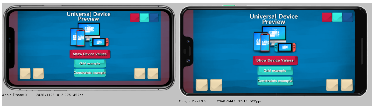
Figure 18: SafeArea constraints. The iPhone and Google Pixel have very different safe area borders.
