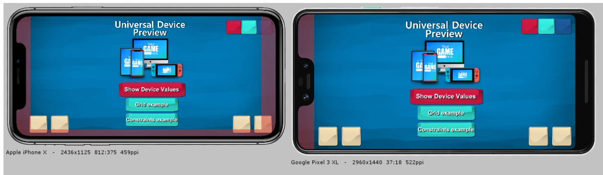
Figure 19: Applying custom constraints to the iPhone SafeArea using a DeviceCustomBorder component. Now the iPhone behaves almost like the Google Pixel. Note that the SafeArea visualization is NOT affected by the DeviceCustomBorder component.
